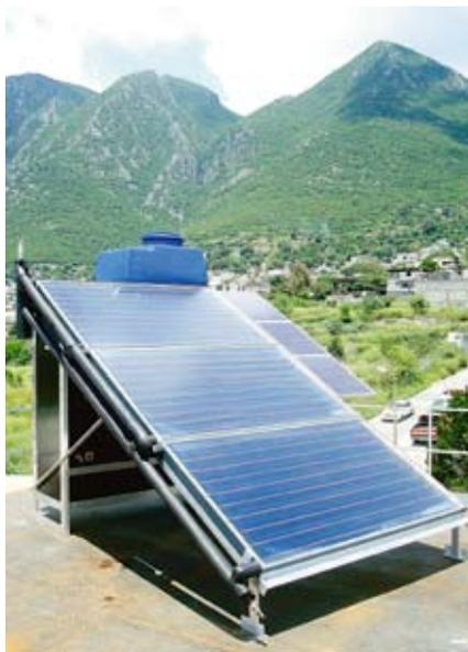
Desalination system set up by the Fraunhofer ISE in Mexico.
